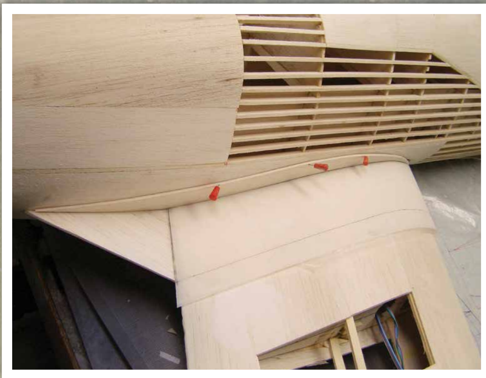
The wing fillet is under construction.
