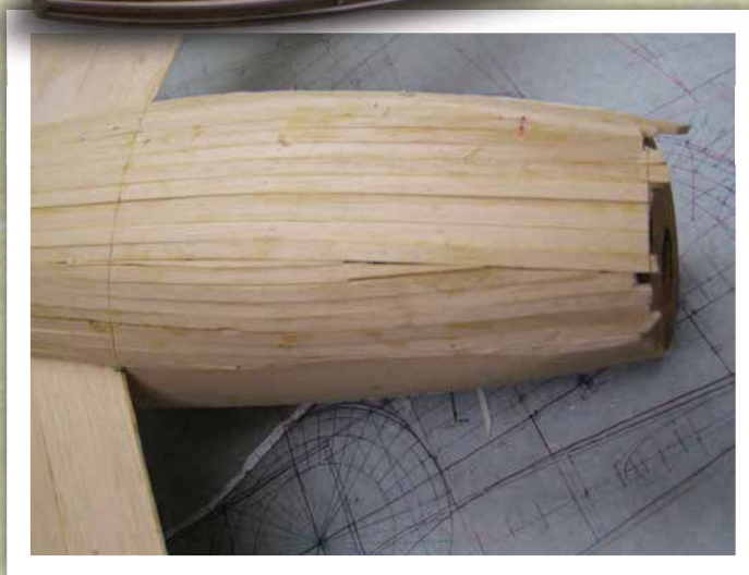
Here you can see the planking on the the bottom of the rear section of the fuselage.
