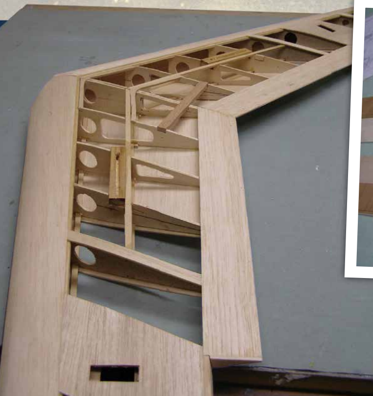
The hardwood blocks for the landing gear are glued to the ribs. The blocks have grooves to accept the landing gear wire.
