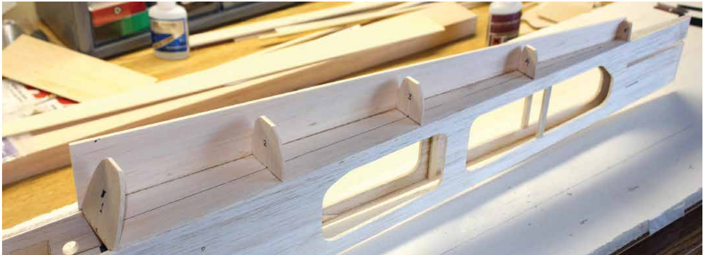
The bottom edge of the right side turtledeck sheeting has been glued to the fuselage side with CA. Next, the outside of the turtledeck sheeting will be dampened with water so the sheeting will better conform to the turtledeck formers, and the sheeting will be glued to the formers with CA.
