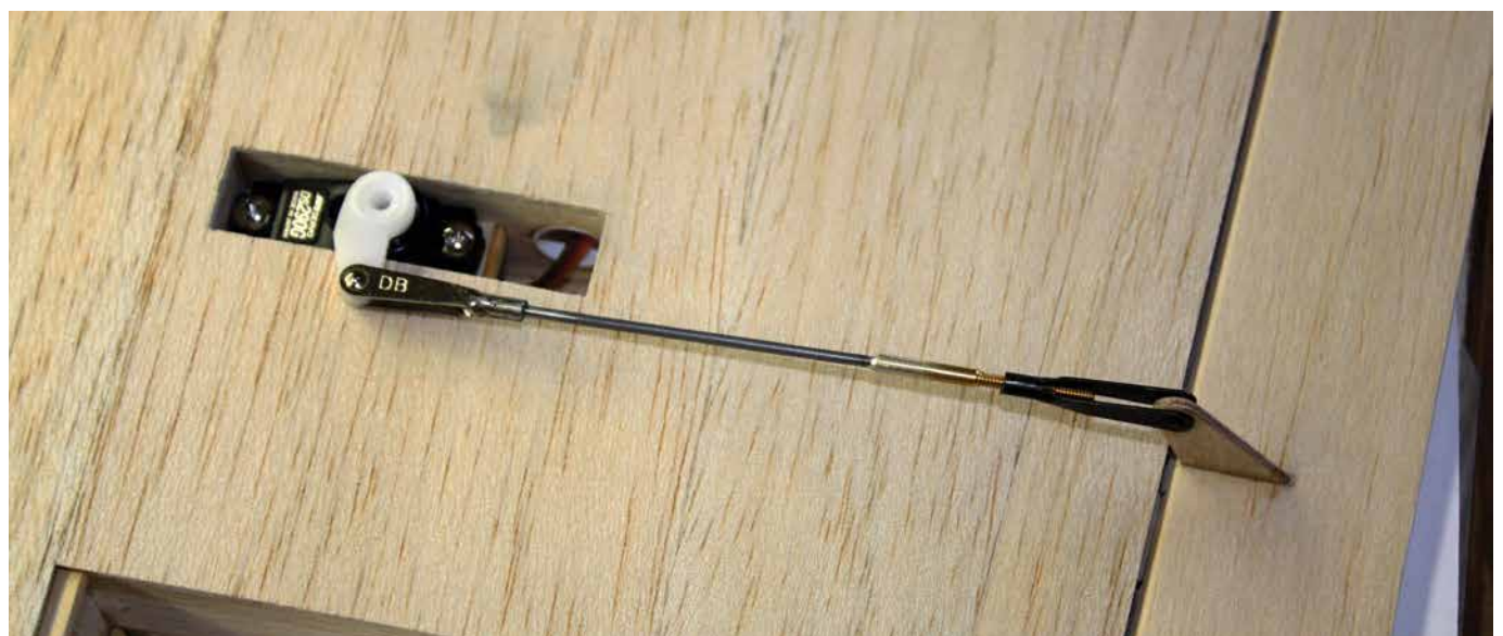
A JR DS290G servo and aileron linkage consisting of a Du-Bro solder Kwik Link, threaded coupler, and Kwik Link on 1/16-inch music wire. The aileron is dry fitted here.
