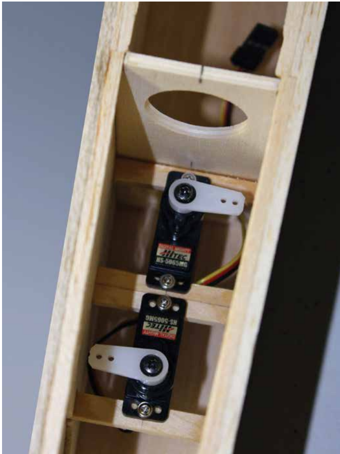
Servo mounts are made from 1/8 x 1/4-inch and 1/8 x 3/8-inch spruce for the Hitec 5065MG rudder and elevator servos. Pushrods will be attached to these servos before the fuselage bottom is glued on.
