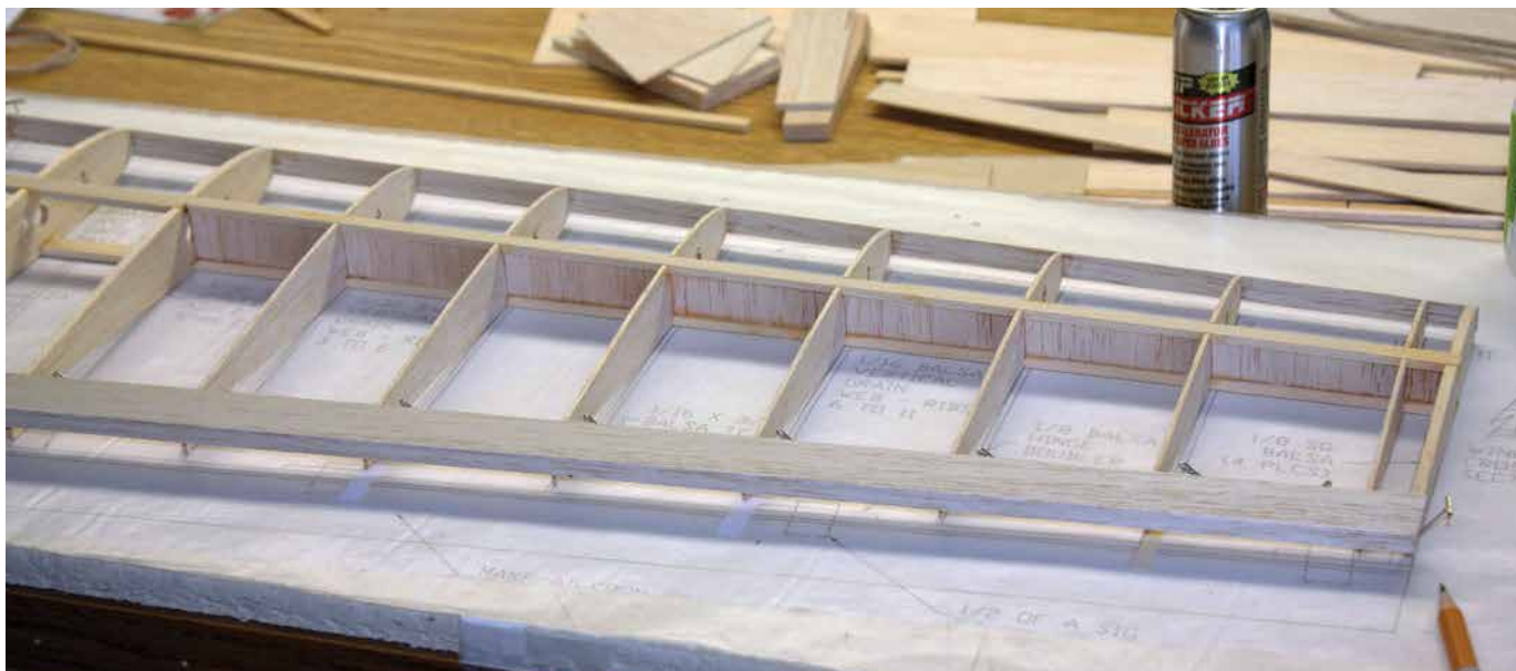
All of the spar webs have been installed except for the first two rib bays where the wing tube resides. The top trailing edge sheet and the sub-leading edge have been glued on.
