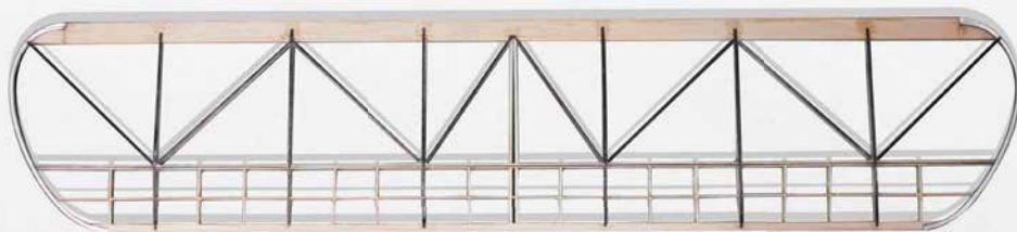
The stabilizer has aluminum-tube tips. Note the carbon-fiber capstrips that have been added to the main ribs and diagonals.
