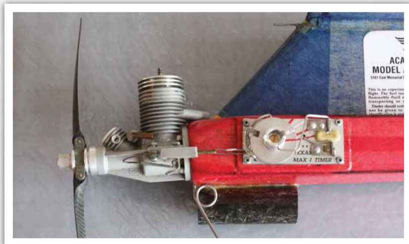
The front end of the model shows the placement of the engine, timer, tank-holder, and nose skid. Note the carbon-fiber folding-blade propeller.
