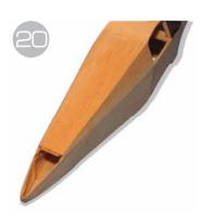
Bevel trim the inside faces of the fuselage top longerons so that the V-tail assembly rests on the top edges of the top longeron.
