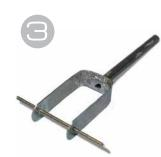
The finished nose strut has a .030 brass wire axle. Solder the axle ends when the nose wheel is in place. The tubing slips over .045 music-wire strut. CA holds the tubing to the strut.
