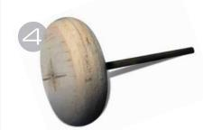
This laminated balsa wheel was turned on a Dremel tool. The 3/32-inch diameter brass tubing is cut off after turning the wheel. Paint it flat black. Add silver paper or Styrene hub
