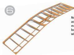
Note that the center section ribs are notched to accept the 1/32 aircraft plywood main gear leg mounting plate. The .045 music-wire struts are bound to the plywood with 28-gauge soft brass wire. CA glue secures everything.
