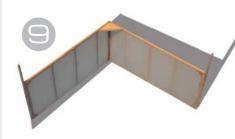
Do not assemble the V-tail until after the two halves are covered with tissue. Note the 3/32 sheet balsa angle attached to the LE of the V-tail. The balsa angle ensures a correct V dihedral angle.
