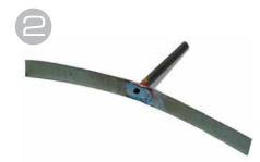
Solder the flared end of the 3/32-inch tubing to the .015 brass sheet.
