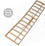
Wing construction could not be simpler. Strong and lightweight, it will hold up to first flights. The tip ribs are covered with 1/32 soft balsa sheet.
