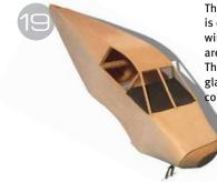
The fuselage sheeting is complete. The three windshield supports are 3/32 strip balsa. The instrument panel glare shield is black construction paper.
