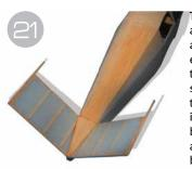
The top edge of the 3/32 angle gusset at the V-tail assembly LE should sit exactly 1/32 inch below the top of the turtledeck sheeting, positioning the LE at zero degrees incidence. Fill the space between the V-tails with a triangular piece of 1/32 balsa sheet. Leave the TE of the V-tail assembly loose to allow shimming in negative incidence.
