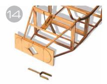
The brass tubing nose strut assembly is ready to slip over the .045 music wire extension. The 3/32 balsa sheet backing at former A facilitates gluing the 1/32 balsa sheet to the cowl cheeks.
