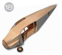
The nose strut radiator housing is built up from soft 1/16 balsa sheet. There is an opening at the bottom rear of the fuselage for attaching the rubber to the rear peg.
