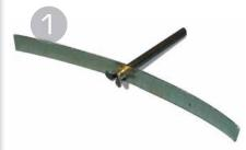
Cut and form a .015-inch brass sheet. Slot and flare the end of a piece of 3/32-inch diameter brass tubing. See the plans for the tubing length and tips for forming the brass sheet.
