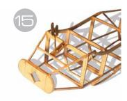
Retain the brass nose strut tubing with gapfilling CA glue.
