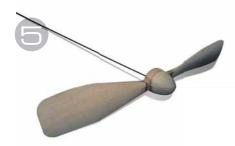
The propeller should be hard balsa, pine, or basswood. Note the slightly rounded blade tips. Start sanding with 50-grit sandpaper and work up to 220 grit. The finished propeller gets a couple of coats of clear dope, then is painted silver with a red spinner. The propeller shaft is .045 music wire. Thread is bound and CA glued to the propeller hub. A Crockett or similar hook is required for winding.
