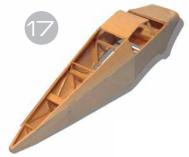
Fuselage sides and bottom are sheeted with soft 1/32 balsa sheet. The 1/32 cockpit top sheeting runs cross-grain.
