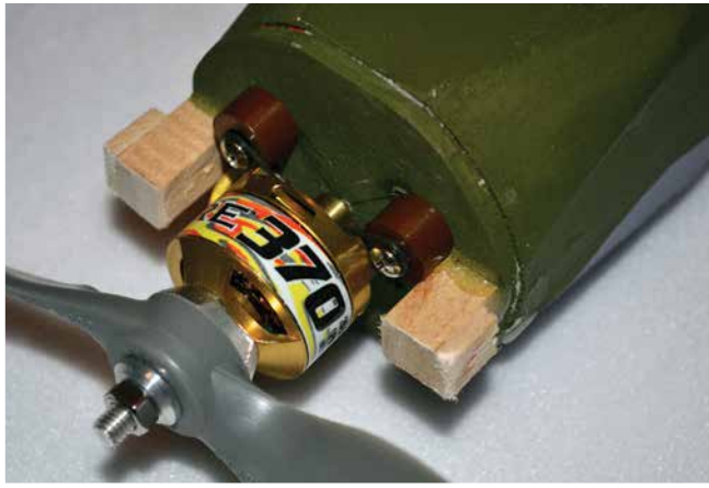
I installed an ElectriFly RimFire 370 motor in my warbird variant of the Parallax. This little motor provides plenty of power. Resist the urge to install larger, heavier power systems.
