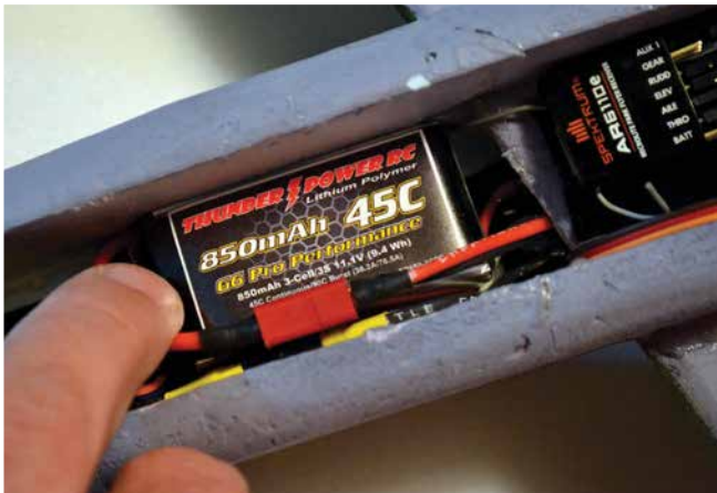
The Thunder Power 3S 850 45C battery is a cozy fit in the fuselage. Velcro keeps it in place. I left the battery area of the fuselage open for easy access and good cooling.
