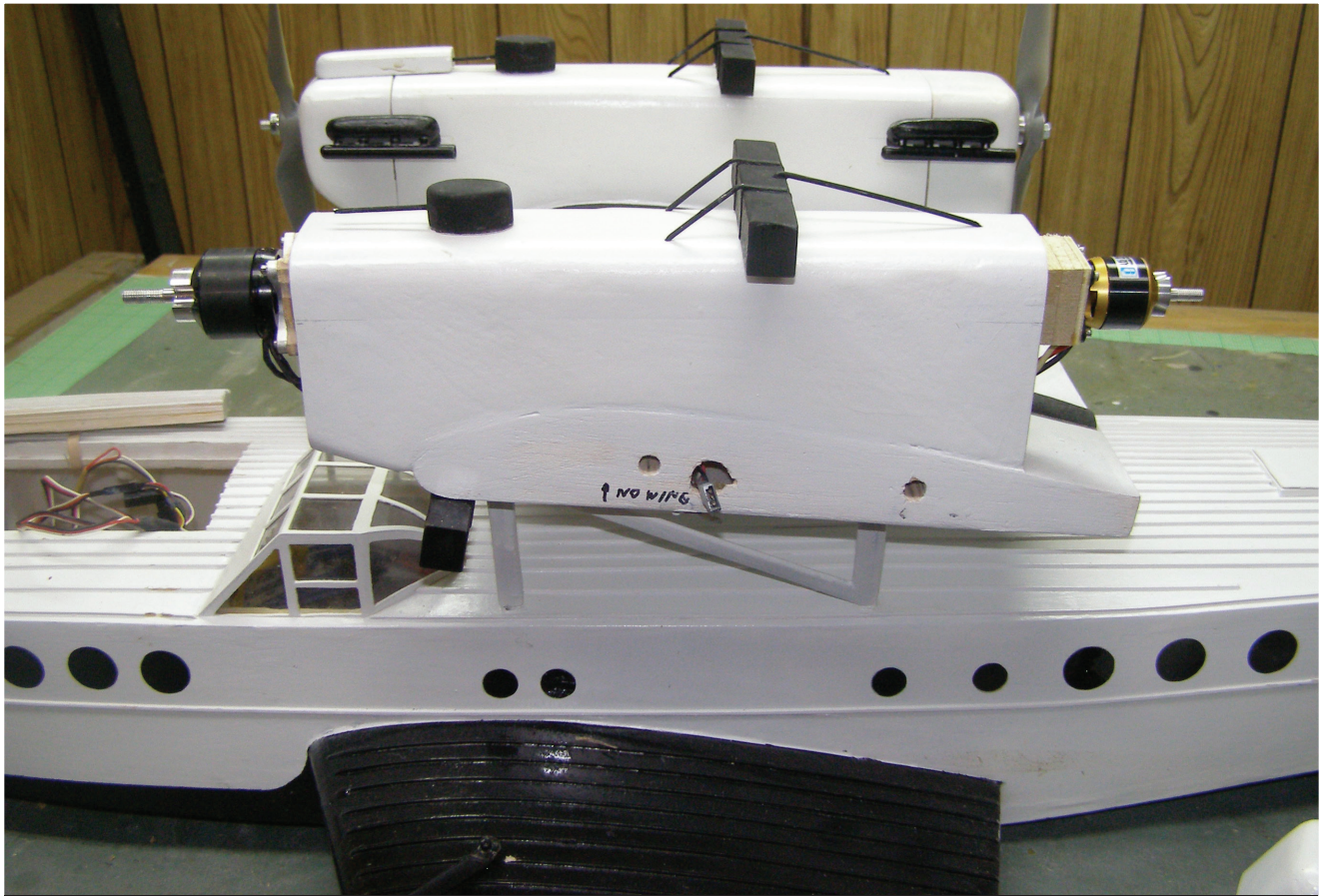
The model is powered by two 2820/14 motors in the front of the nacelles and by two 2212/34 motors in the rear of the nacelles.
