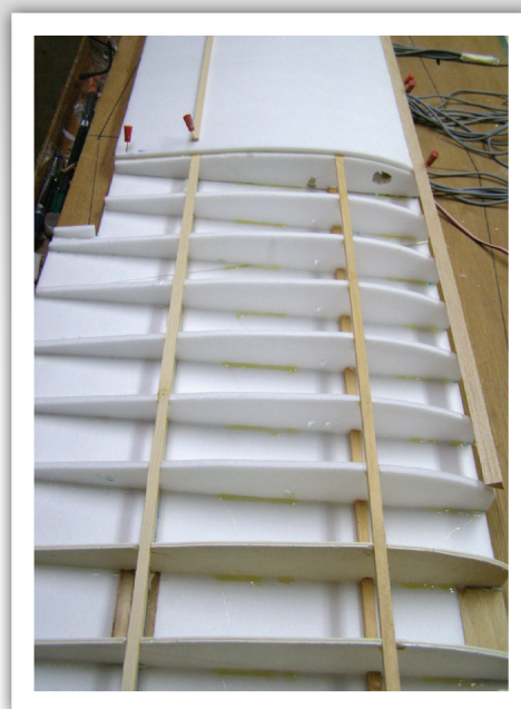
The ribs have been glued in place and top spars glued to the ribs. The top sheeting is being glued on.
