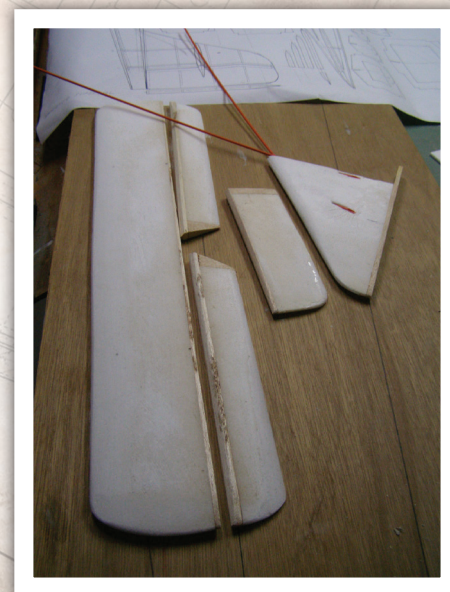
The tail surfaces are 3 / 8 -inch thick. Two 3 / 16 -inch foam sheets are glued together and then sanded to shape.
