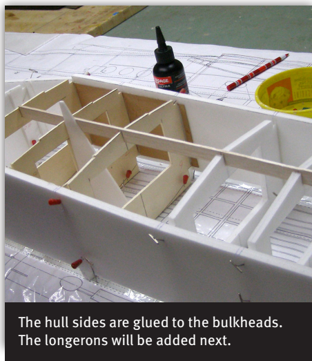
The plywood doublers are glued to the hull sides and the fuselage bulkheads are positioned and pinned to the building board. Notice that the tabs are attached to the bulkheads.
