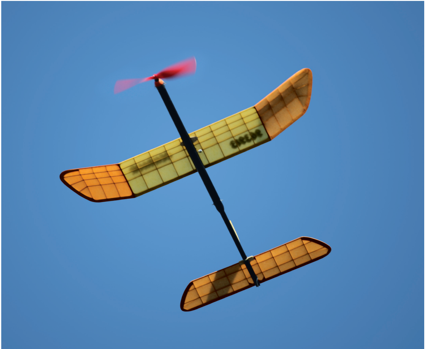
The model is trimmed for a steep spiral climb to the right, which will transition to a right glide turn because of the built-in tailplane tilt.
