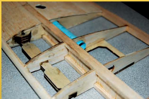
The landing gear blocks can be cut from hardwood or built up from plywood.
