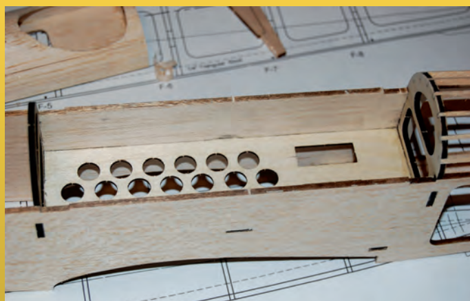
The plywood battery compartment floor is perforated to allow air to circulate, and the cockpit openings allow heat to escape.
