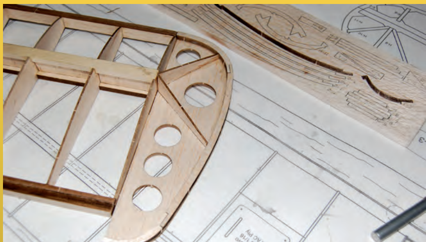
The wingtip can be built-up on the wing or assembled and added to complete it.
