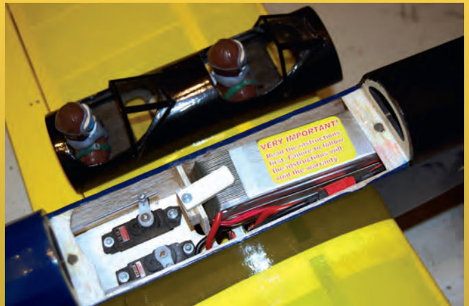
Turnaround time between flights is less than a minute because the hatch simply lifts off. The battery can quickly be swapped.
