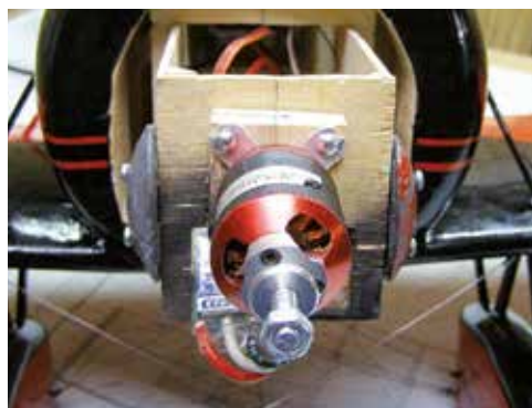
With the cowl removed, there is access to the motor, speed controller, battery, and the receiver. Notice the lead attached to the side of the motor box.
