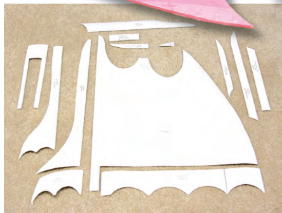
To generate foam marking templates, use pieces of transparent paper and copy the main components from the plans.
