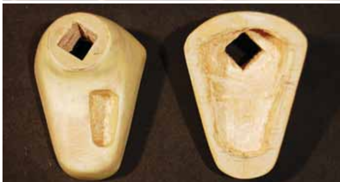
The exterior and interior of the balsa nose block looks like this before painting. These are held to the fuselage with magnets.
