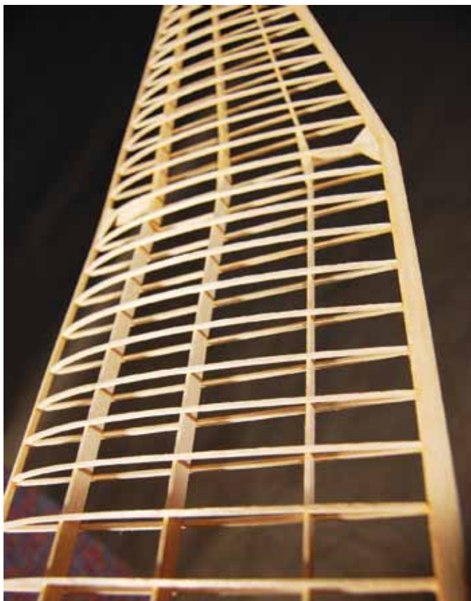
The wing uses a sliced-rib construction that is light but strong. Use a thin plywood template to slice the ribs.
