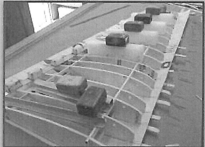
Below right: Weights and shims were used to bond the ribs to the bottom sheeting. The polyurethane glue sets slowly, allowing plenty of time for adjustments.
