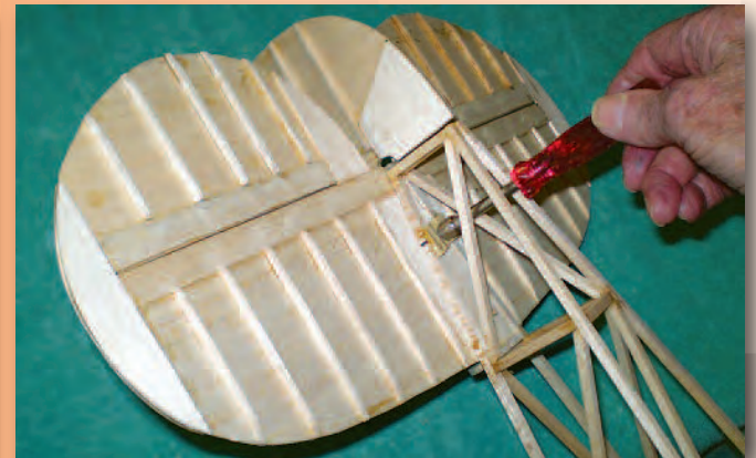
The tail assembly is bolted on or removed with a socket wrench inserted through an opening in the bottom of the fuselage. The whole assembly is quite rigid and allows for removal if needed for adjustment or transport.
