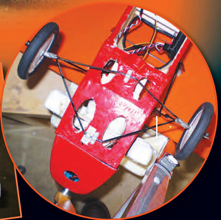
The landing gear is made from music wire and attached with nylon bolts to the plywood landing gear plate. Note the openings, which save weight and provide cooling vents.
