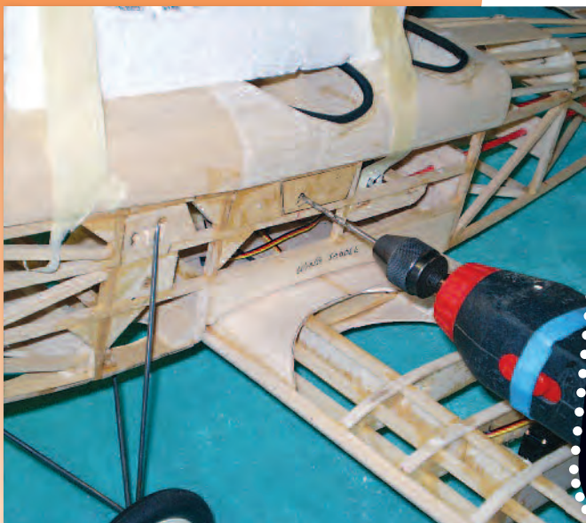
Now that the correct positions of the cabanes have been determined, you can drill their holes in the plywood support blocks.
