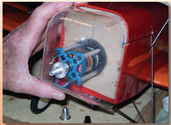
The cowl is vacuum-formed plastic. It is held to the firewall with two magnets mounted in a frame around the inside back of the cowl.
