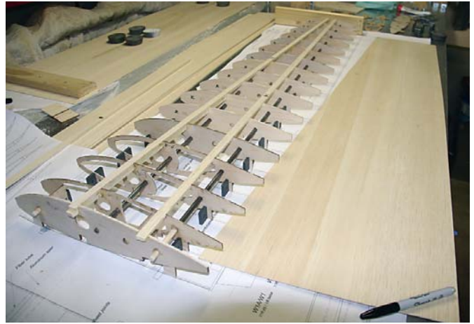
A laser-cut parts pack is available from Home and Hobby Solutions (Jeff Petroski). A fixture holding 1/4-inch metal rods aligns the ribs located over the plans sheet.
