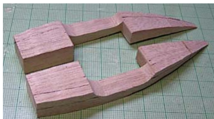
Right: Assemble nacelle parts with the kind of wood glue that is easy to sand. These should fit the wing sections as tightly as possible.
