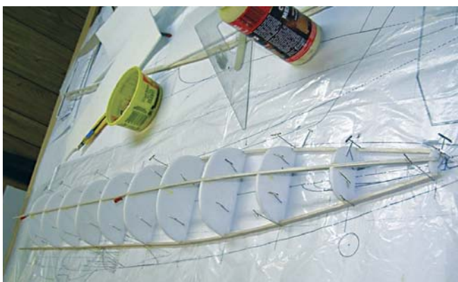
As does the lower half, the fuselage top section and longerons build flat on the table. All formers are foam.
