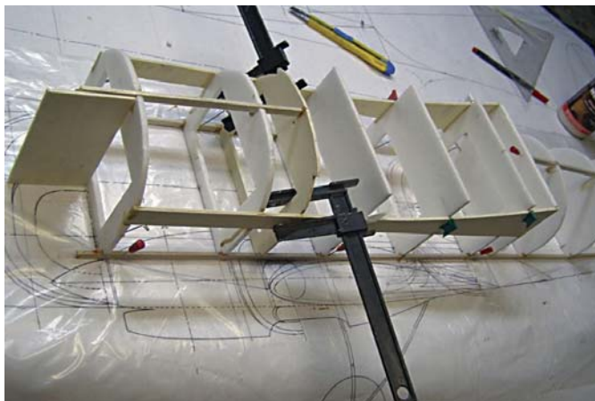
Bottom formers and longerons are shown. Formers at lower stress areas can be made from lighter closed-cell-foam sheet.
