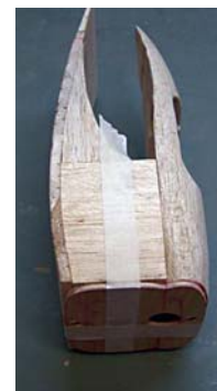
Right: Assemble nacelle parts with the kind of wood glue that is easy to sand. These should fit the wing sections as tightly as possible.
