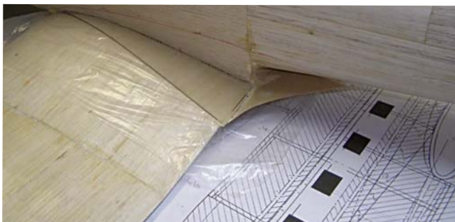
Above: From the dividing line on top and the TE at the bottom, the fuselage is covered with 1/8 x 1/4 balsa planks. The wing fillet base is glued to the fuselage.
