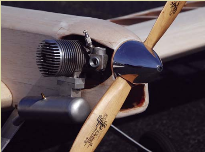
The cutout is large enough through which to pull out the Moki 1.80. It is mounted sideways, so that the standard muffler tucks in tightly against the fuselage. Balsa blocks are faired into the spinner.
