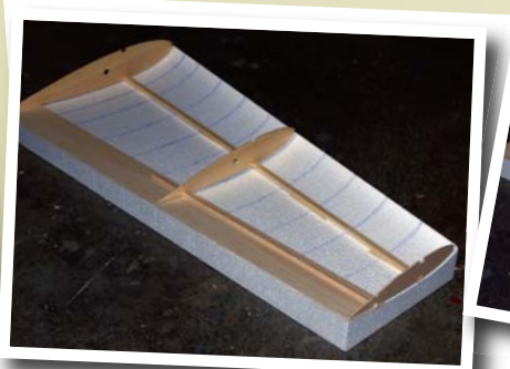
The wing assembles into the cradle. The lower spar, lower TE planking, and first few ribs are shown positioned in the fixture.
