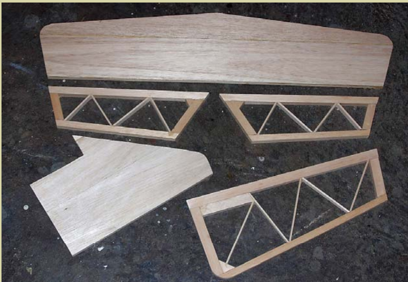
All cut balsa and plywood parts needed for fuselage construction are shown. Today's modeler has to pay through the nose for good material, but we build for the fun, not the price.
