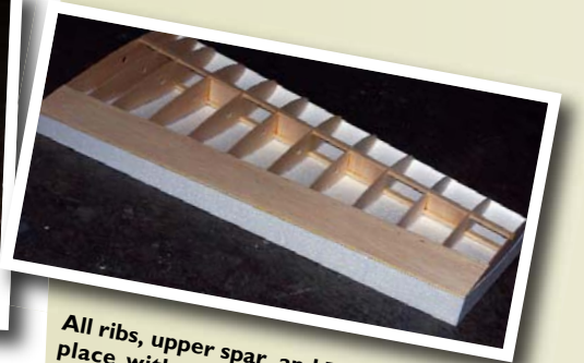
The wing core itself is cut apart at rib location positions, ready to be used as patterns for balsa ribs. Because ribs will be cut from these foam patterns, they will fit perfectly in the foam fixture.
