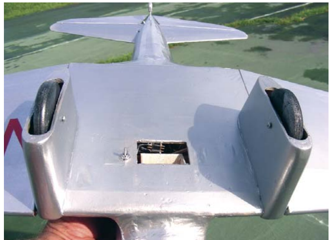
The battery compartment is a sloped box, accessible from the bottom of the fuselage. Notice the on/off power switch. Do not transport this model with the Li-Poly battery installed.
