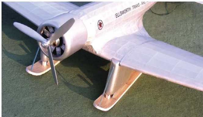
Models this size seldom do a good job of landing or taking off from grass, but the version with skis seems to land better on grass than the wheeled version.
