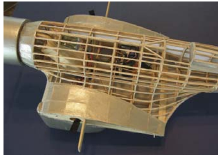
The fuselage is built in half shells. Then those are mated, creating a nice, light framework. Some stringers in the wing-fillet area take on difficult curves; use light balsa soaked in water to install those.
