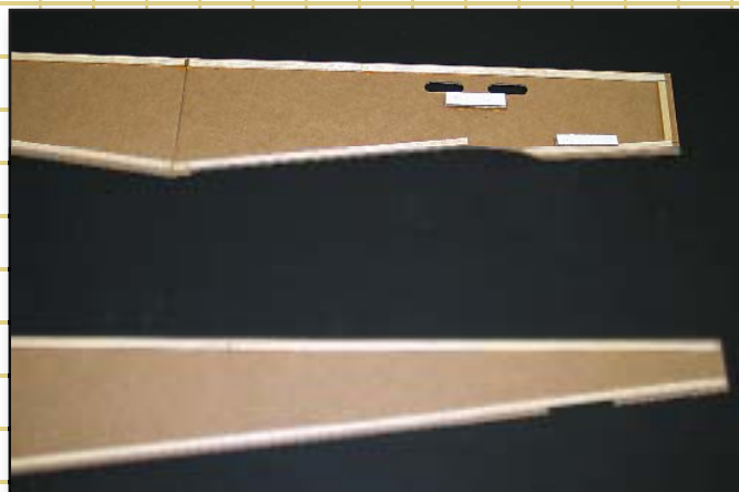
Flat fuselage sides are lined with balsa strips and have cardboard supports for bellcrank and fuel tank mounting.
