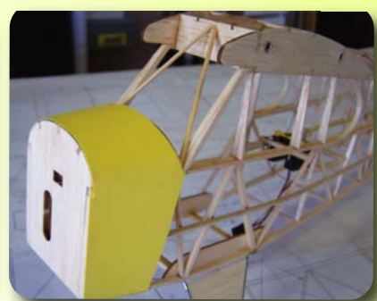
A boot cowl is made from file-folder paper and adhered with white glue. The paper takes covering almost as well as wood does and simulates aluminum skin.
