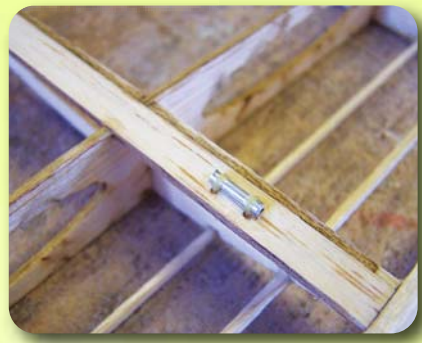
The \frac{1}{16} -inch-OD aluminum-strut retention tubes are lashed to the wing panels with Kevlar thread and secured with a drop of thin CA.
