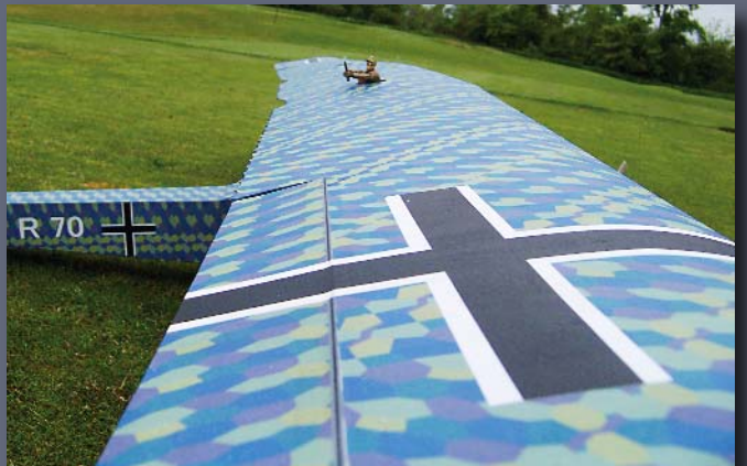
This five-color lozenge pattern is a modified version of one that Jim found on the Internet. He printed it on tissue and then applied it over Solite.
