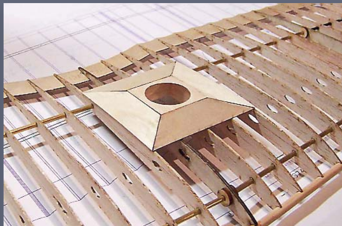
The top wing has two turrets built from \frac{1}{8} balsa and covered with \frac{1}{32} plywood.
