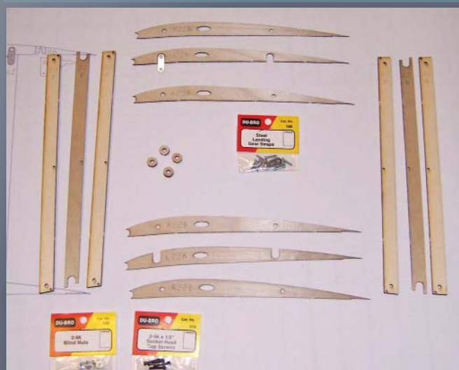
Laminated interplane struts are attached to laminated ribs using Du-Bro straps. These provide a secure and easy method of attachment.
