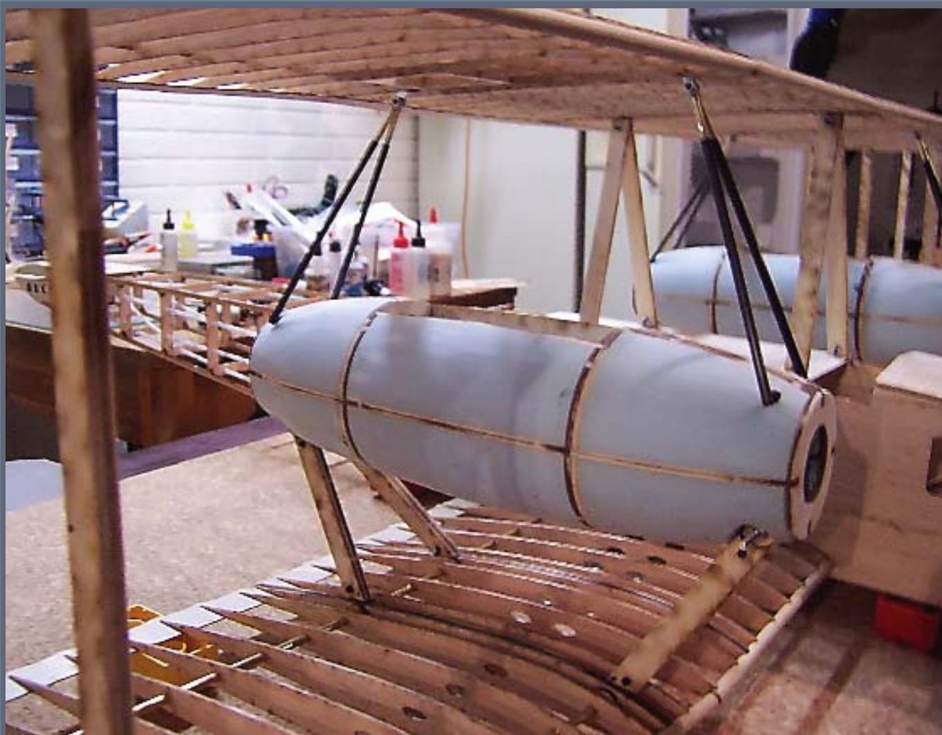
Blue foam has been sanded to shape to form the engine nacelle. It is supported with light plywood and carbon-fiber rods.
