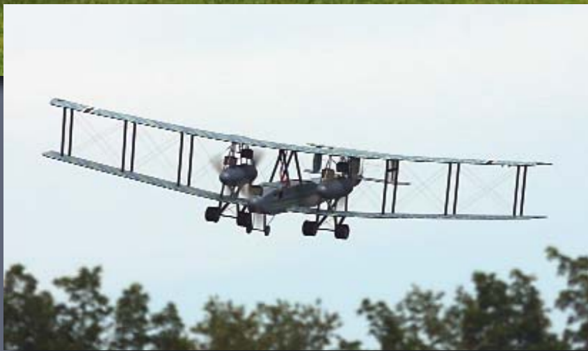
Right: The five motors put out approximately 64 watts per pound. The amount of drag on this large bomber requires that it be at full power throughout the flight.
