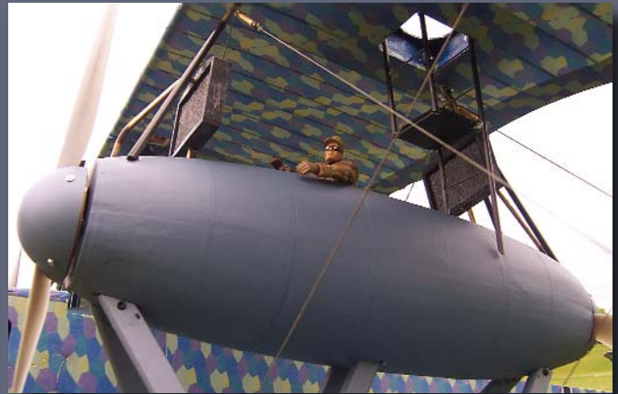
This shows the externally mounted radiators; each of the five motors has one. The mechanic is standing in the access opening that made in-flight repairs possible on the full-scale aircraft.
