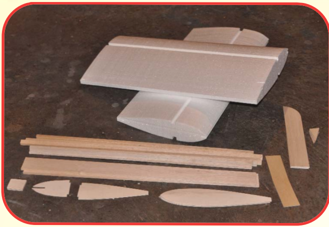
Wing parts including cut foam wing cores and all necessary balsa and plywood parts.
