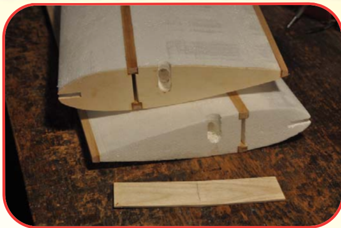
Root ends of the two wing panels, showing the center plywood rib and holes through the foam cores for aileron servo cables. The plywood dihedral brace is used to support the wing joint.
