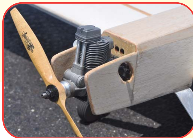
A Magnum .70 four-stroke engine is located on a molded composite radial mount. The hole in the cowl side provides access for the needle valve and choke lever.
