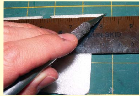
Above: To create hinge bevels, use a ruler and a sharp #11 X-Acto blade. Hold the knife at a 45° angle and pull it slowly through the material.
