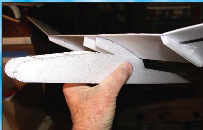
Two center wing ribs fit snugly inside the two fuselage sides. Align the wing with respect to tail surface, set in the proper incidence angle, and apply CA cement. This is an easy process.
