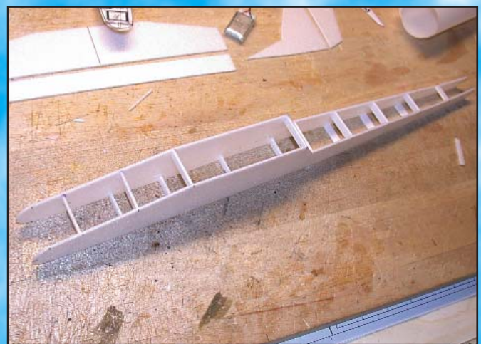
A fuselage assembly fixture was made from \frac{3}{16} balsa sheet. It follows the top view of the fuselage. Both Depron foam sides are pinned to this fixture. Partial formers are added above and below the fixture.
