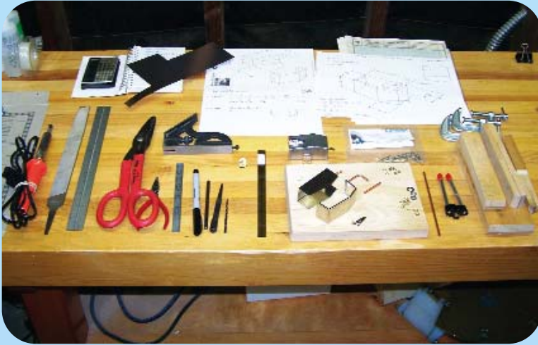
This complete set of tools will help you build a good tank. Wood blocks are bend-forming tools. One thing is missing: the small propane torch used to anneal the copper tubing before bending.
