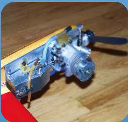
The ShyFox is fueled through a uniflow line via a fitting attached to the top engine lug; black tubing is the seal. The alligator clip is pressed during fueling, opening the overflow line. Since the clip has minimal spring force, thin-wall surgical tubing is used.
