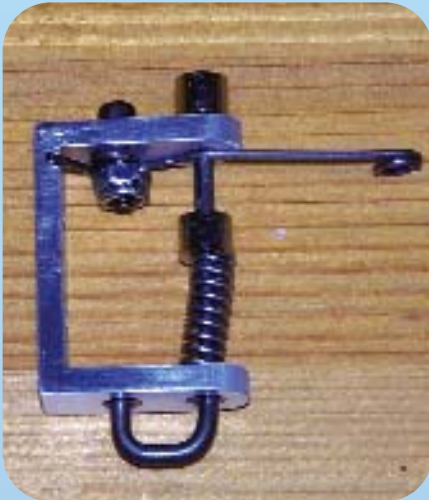
Modified "Dirty Dale" small shutoff. The left edge is screwed to the engine plate. The fuel line goes through the pinch aperture at the bottom, which has an adjustable spring force and can be used on soft \frac{3}{32} -inch-diameter silicone tubing.
