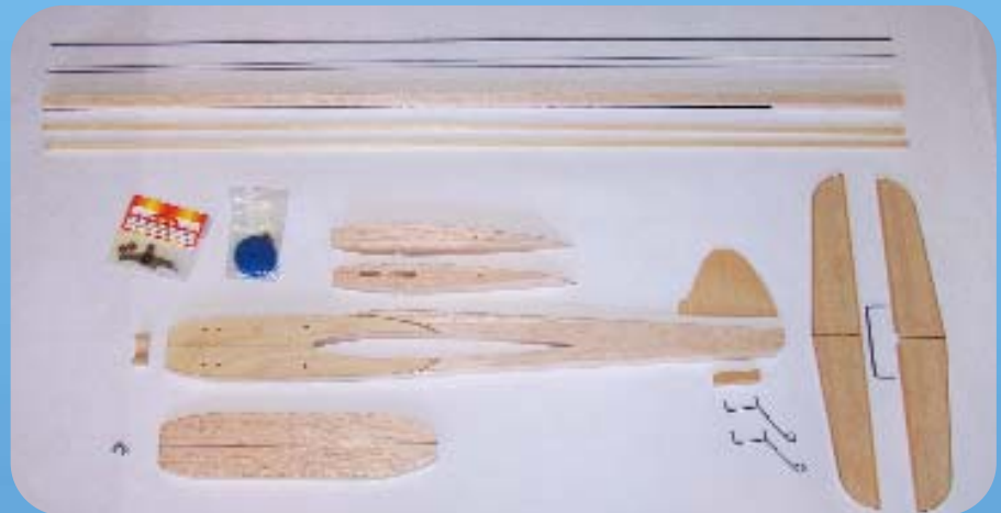
Major airframe parts in the early assembly stage. Use accurate layout lines on all pieces, and make sure centerlines line up during each step. The Fox bellcrank is the way to go.
