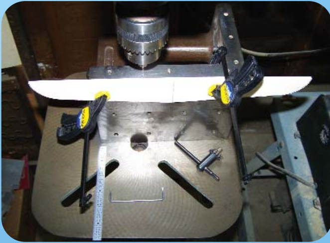
Elevators are ready to drill for the joiner wire. This method provides much control and accuracy. Use a \frac{3}{32} -inch-diameter drill, but go only as deep as the joiner arms to avoid breaking through when shaping.
