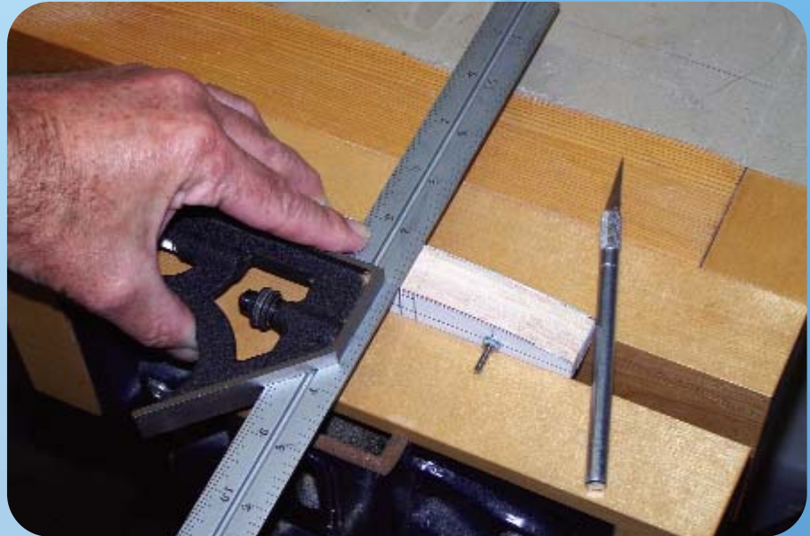
After ribs are shaped, cut spar notches. The template establishes the location and a square aligns the cut; a vise leaves one hand free to hold the knife.
