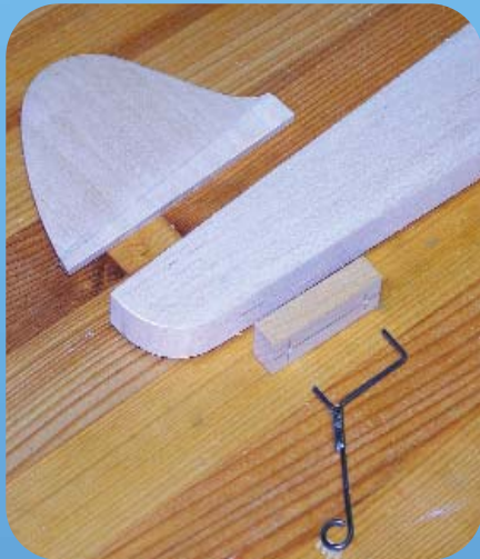
Cut these fuselage features before tapering it to improve accuracy. The tail skid is assembled from two pieces of music wire, wrapped with copper wire and soft-soldered.
