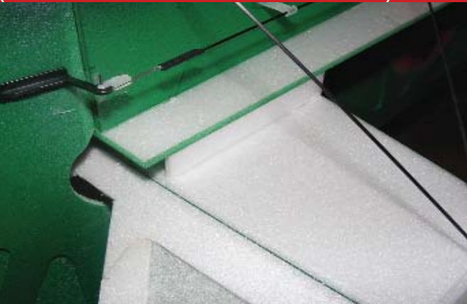
The stabilizer was purposefully located above the thrustline. Notice the rudder control horn, how the pushrod is installed, and the hinge bevel angle.
