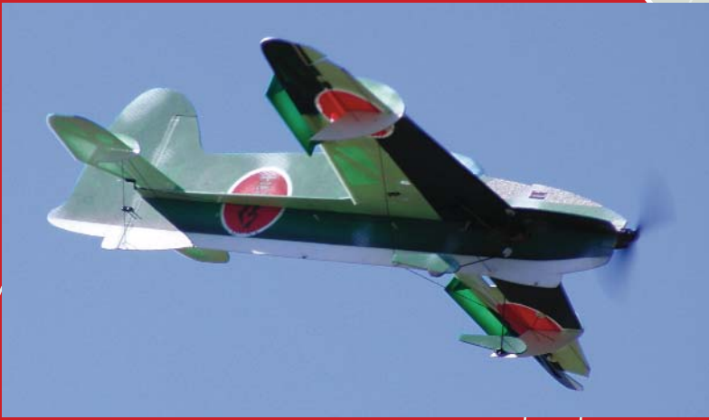
Setting up for an approach. This model has lots of fuselage side area; this is the main reason why minimal rudder is needed in knife-edge flight.
