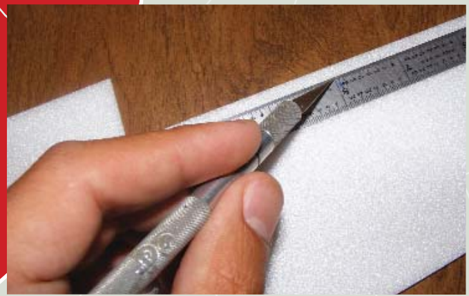
You can hinge the ailerons, elevator, and rudder with a ruler and a sharp X-Acto blade. Bevel the bottom of the control surface so that the model can be top-hinged.
