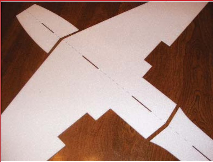
The front and rear horizontal fuselage pieces are ready to be glued to the wing. Take time when cutting the foam components, to ensure the utmost accuracy.
