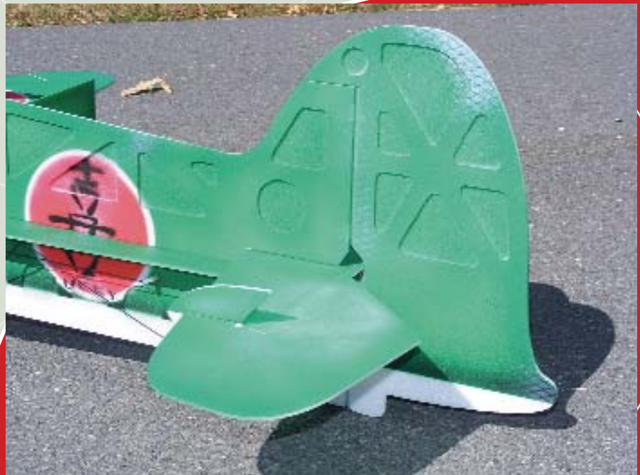
SFGs are used on both the wing and the horizontal stabilizer. Carbon-fiber crossbracing on the tail was added later, to keep the fin straight.
