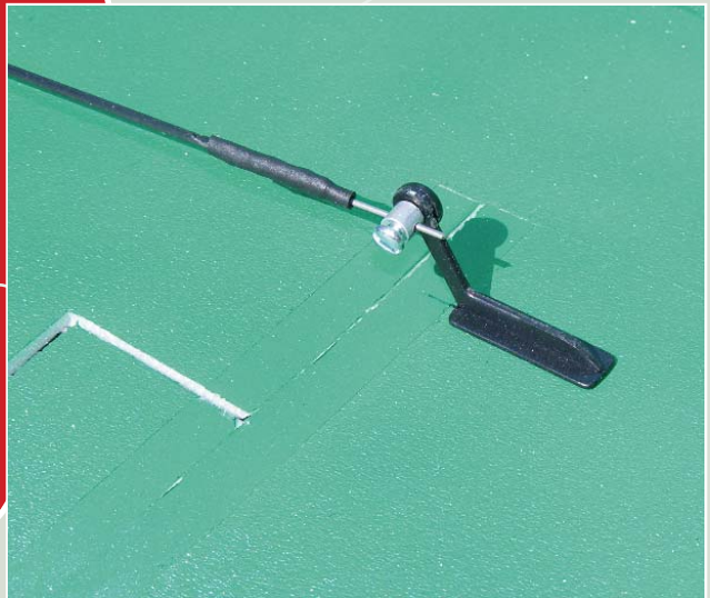
The control horns used are a modified version of the standard Du-Bro variety. The aileron carbon-rod linkage is glued to the .032 wire, wrapped with Kevlar thread, and completed by sliding heat-shrink tubing over the entire assembly.
