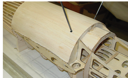
The landing gear uses conventional music wire and nylon mounting straps. The bottom of the fuselage is finished off with \frac{1}{16} balsa sheeting.
