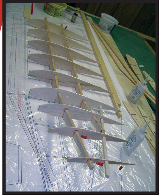
Above: All ribs are cut out, and the main and auxiliary spars are in the process of construction. The wing is built with a left and right half.
