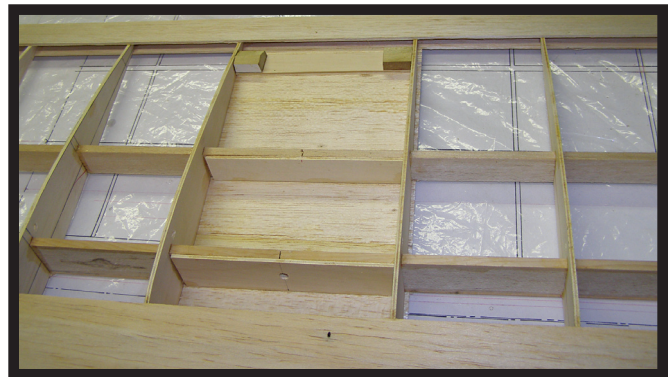
Above: The top TE is glued to the ribs. The hardwood landing gear block is glued to the ribs. Pre-drill the block for the 5/32-inch-diameter piano wire.
