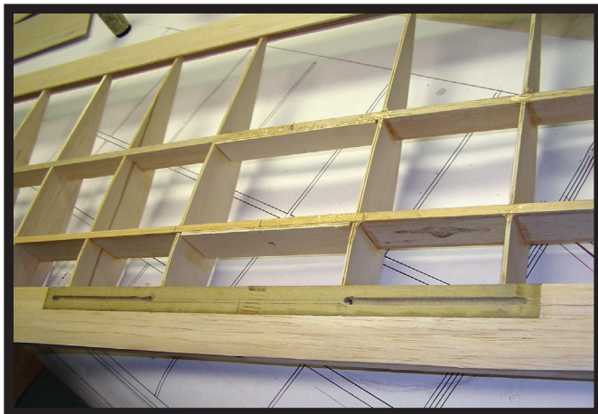
Above: The top TE is glued to the ribs. The hardwood landing gear block is glued to the ribs. Pre-drill the block for the 5/32-inch-diameter piano wire.
