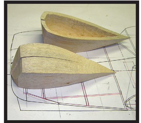
The cheeks for the engine cowl are fabricated from balsa blocks. Making them identical can be tricky; take your time and use the plans as a template.
