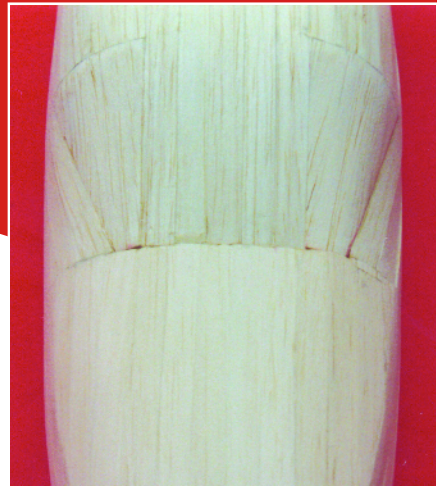
The compound curves will be smoothed with lightweight filler. Each plank is custom-fit with tight joints.
