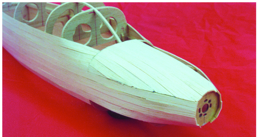
Do the planking as neatly as possible (as shown), so that the amount of sanding needed for the 1/16 balsa is minimal. Four planks run uninterrupted from tail post to motor mount.
