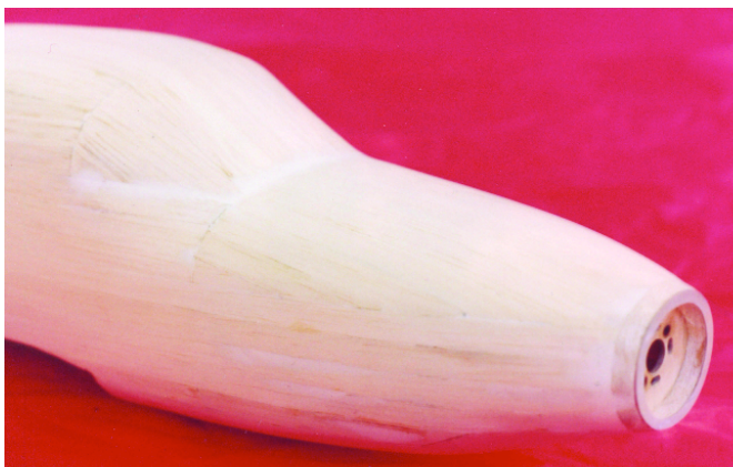
Lightweight balsa filler (a balsa-colored type was used on the Lancair) hides the seams and rounds the corners.
