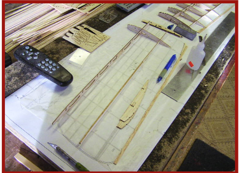
The wing assembly begins with all spars, ribs, and TEs glued together over the plans. Once the basic right wing is framed, the left wing is assembled to the same point.
