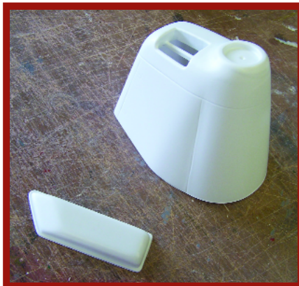
The vacuum-formed cowl and oil tank are trimmed from their carrier sheets, and their edges are sanded smooth.
