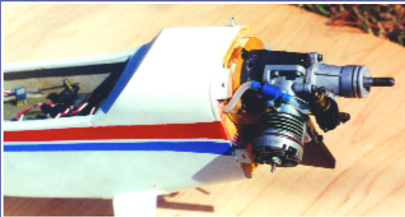
The author employed a universal muffler (no longer available), but others can be used. The .25 engine used in the prototype flies the Midsport 20 nicely.
