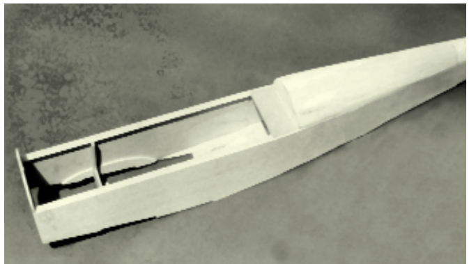
On the finished basic fuselage structure, the firewall (F-1) has been glued in place and holes have been drilled for the engine mount and 4-40 blind nuts. The rear top deck is temporarily in place.
