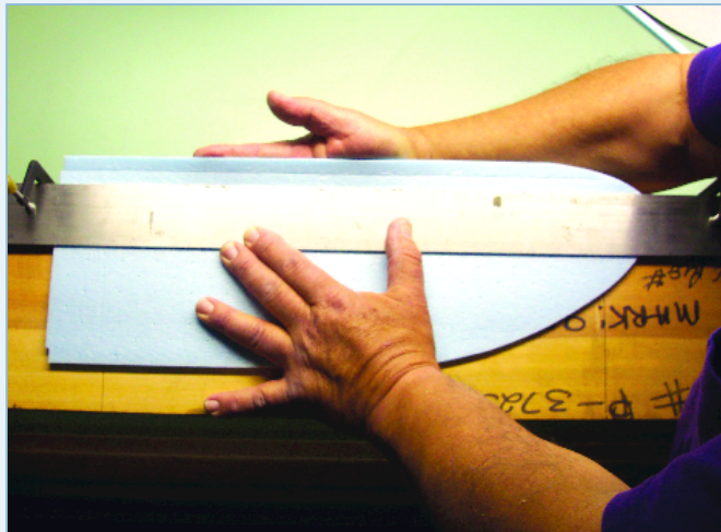
Create each wing panel's airfoil with a metal ruler and crisp table edge. Bend the LE to shape one crease at a time.
