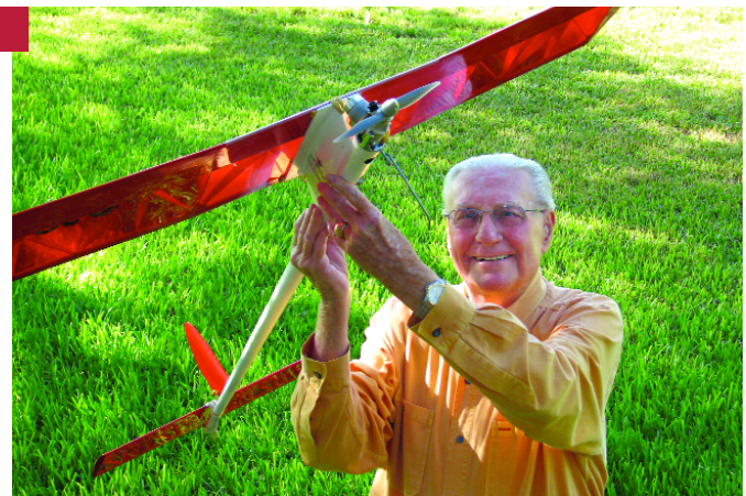
The author holds his Super Marval under a shade tree while the Texas sun blazes. The wing and stabilizer are covered with light iron-on film.
