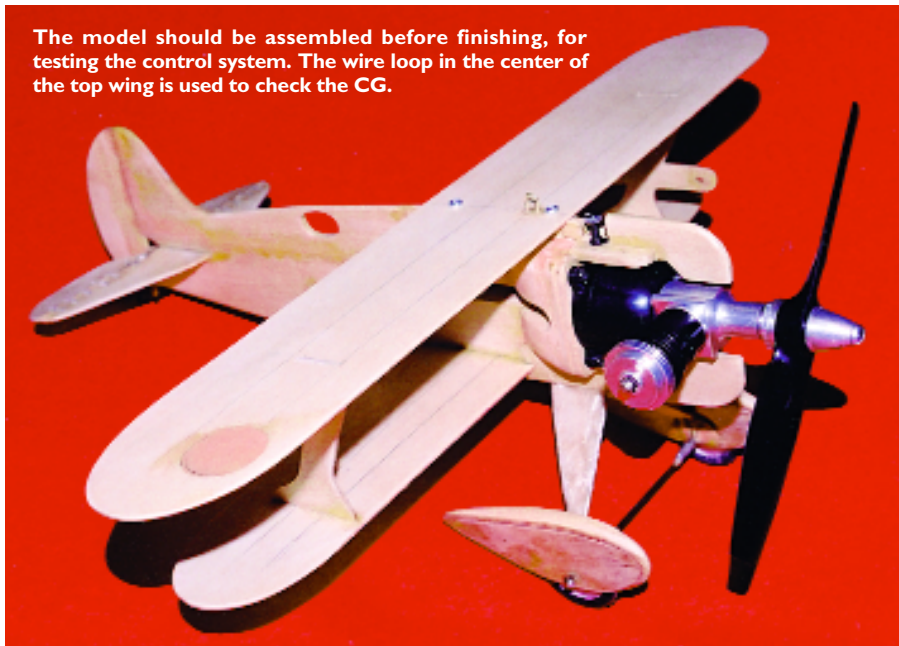
The brass ram air intake is the secret to good 1/2A engine performance. It's shown epoxied to the 1/4 plywood firewall.
