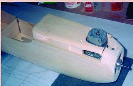
Above: The He 100D is centered around the SuperTigre .51 engine's power capabilities. Choose the balsa filler blocks carefully to save weight.
