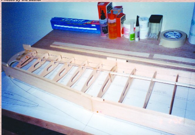
Wing construction uses 1/4 x 2 balsa sheet on edge over the plans; it doubles as building fixture and LE and TE. Hal deBolt pioneered this wing-building method.
