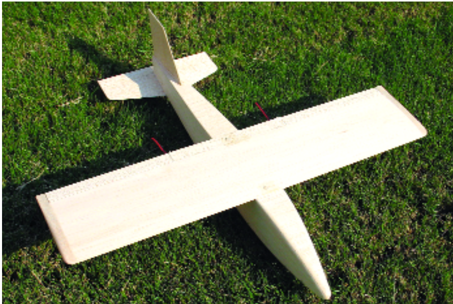
The completed airframe is ready for dope or a different lightweight finish. Power leads exit the rear of the motor nacelles, to be soldered to the motors after the model's finish is applied.
