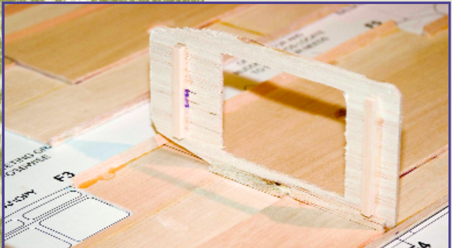
Former F4 is glued in place on the right fuselage side; \frac{1}{4} square balsa reinforces F4 crosswise. Balsa triangle stock reinforces the glue joint between F4 and the fuselage side. Notice that the top of F4 has not been glued to the side yet.
