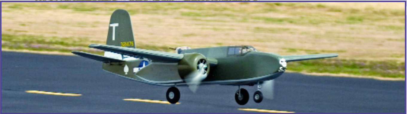
For easier takeoffs, program the nose-wheel steering to be less effective by setting up a mix switch. The A-20 comes up to speed quickly on smooth runways.
