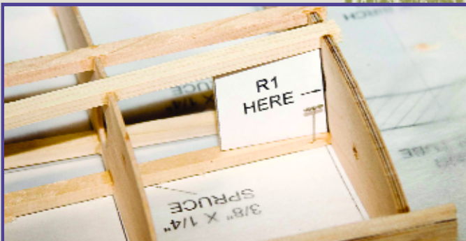
Rib R1 is glued to the upper and lower wing spars at the correct angle using the template cut from the plans and glued to a piece of scrap plywood.
