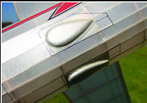
The fuselage, wing, and tail surfaces were covered with white Japanese tissue followed by a light coat of aluminum dope—a mixture of clear dope and aluminum powder—sprayed, with an old-fashioned artist's atomizer.
