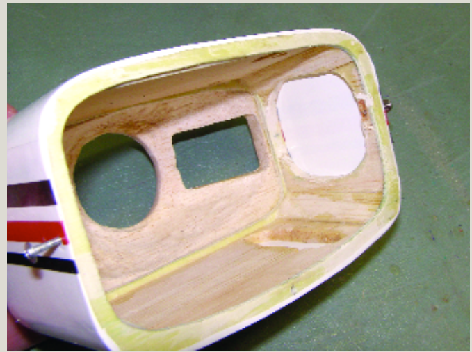
The balsa-and-plywood cowling can be built with or without the option to explore power sources. The power pod is mounted high enough to suit a 13-inch propeller.
