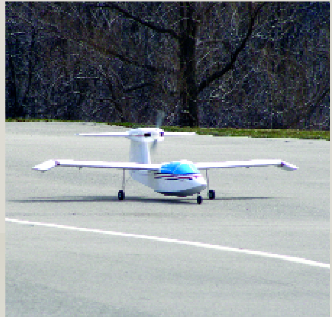
As shown on the plans, removable fixed wire landing gear can be attached to the model for grass or paved flying days.
