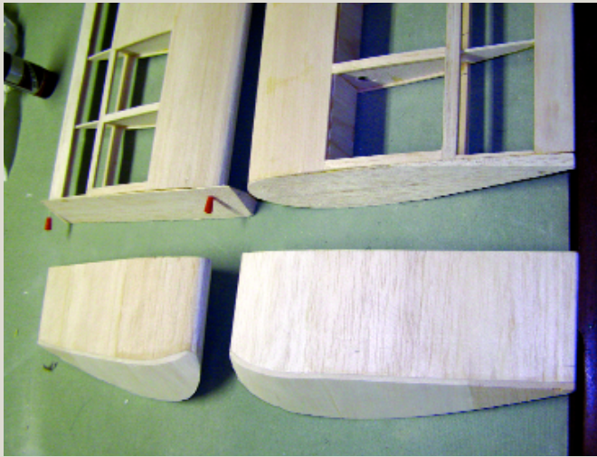
The wingtips are made, showing the use of a balsa wedge to get them at the right angle. The builder has the option of omitting this wedge and angling ribs W11 and W12 instead.
