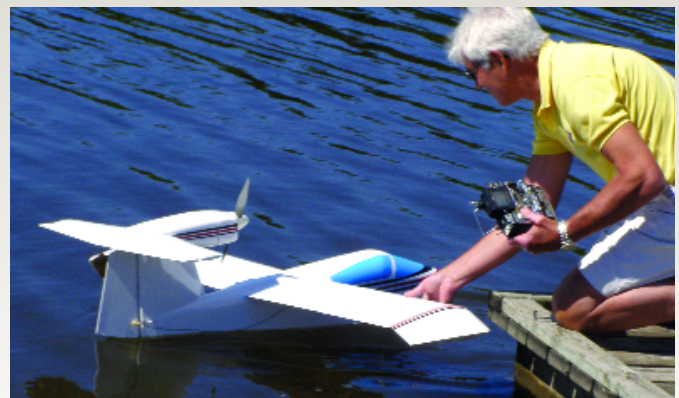
Laddie clears the model from the dock for taxi. The water rudder is optional and adds authority to water steering, but it requires careful management on takeoff.
