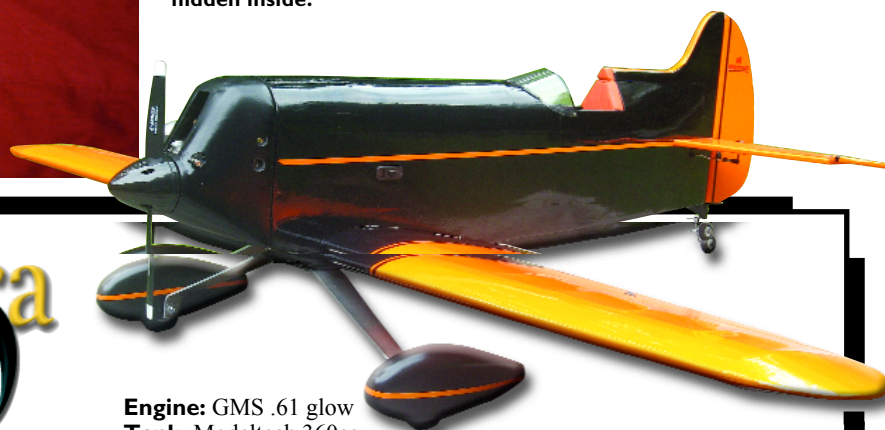
Left: Build the cowl from wood or purchase the fiberglass version from Fiberglass Specialties. The mounting screws are hidden inside.
