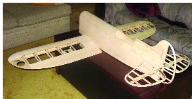
Above: The completed one-piece wing is mounted with dowel pins and nylon bolts. The light tail structure is designed to keep the weight mass balanced on the recommended CG.
