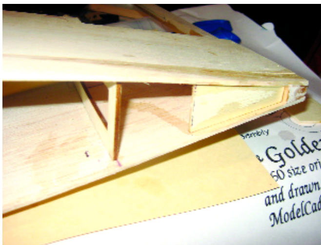
The tail-wheel mount area is supported by a \frac{1}{8} plywood plate. It's recessed to allow room for balsa, which will be sanded flush with the fuselage sides.
