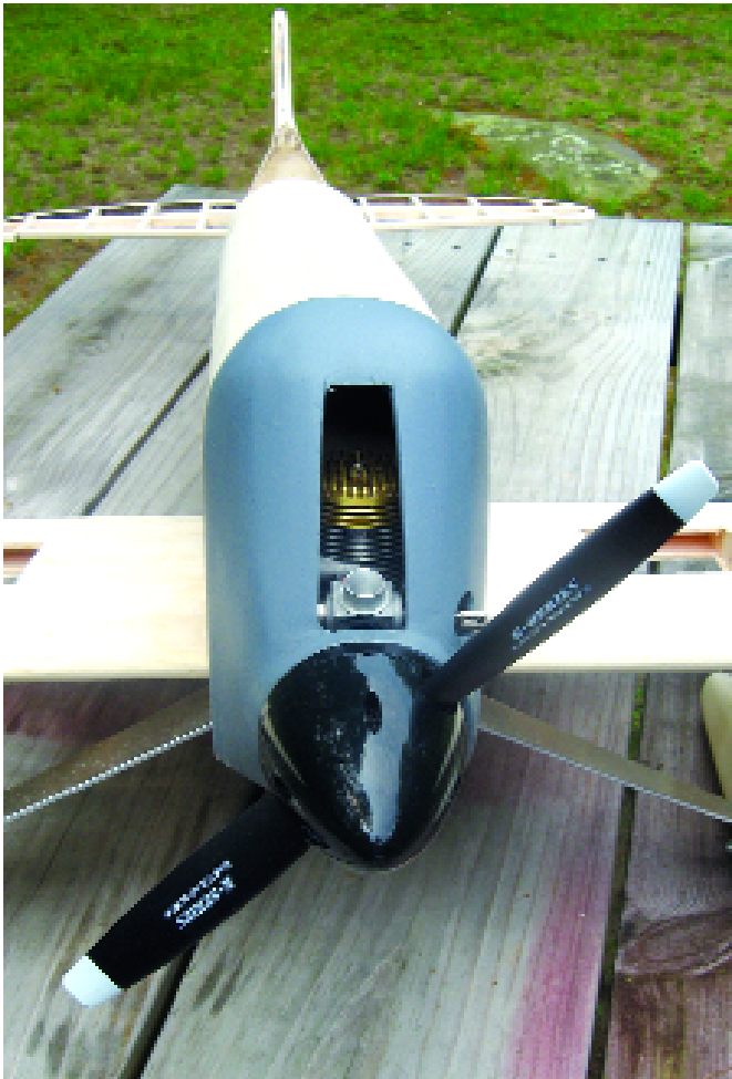
The GMS .61 two-stroke engine hides inside the spacious cowl. A four-stroke .82-1.00 would also fit this model neatly.
