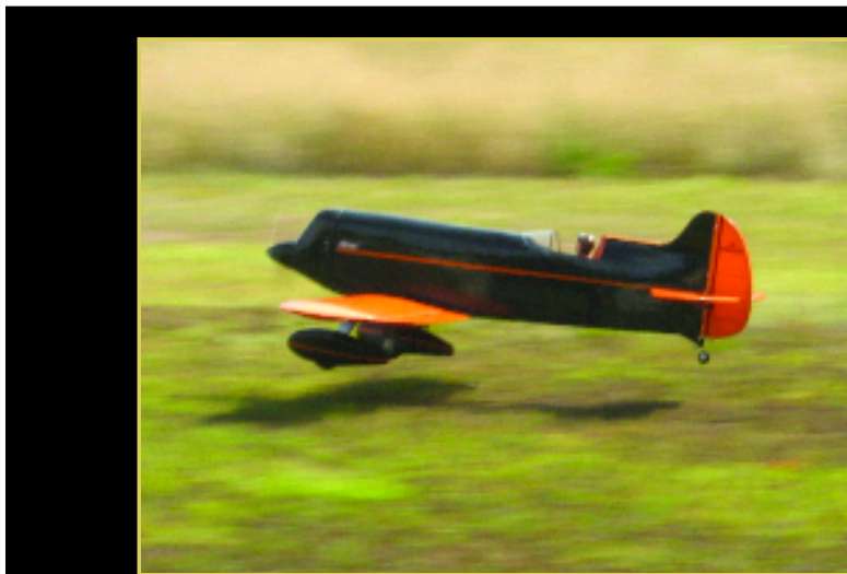
After a full-power run of roughly 50 feet, the model lifts off smoothly. The wide-track gear absorbs many of the bumps in the grass.
