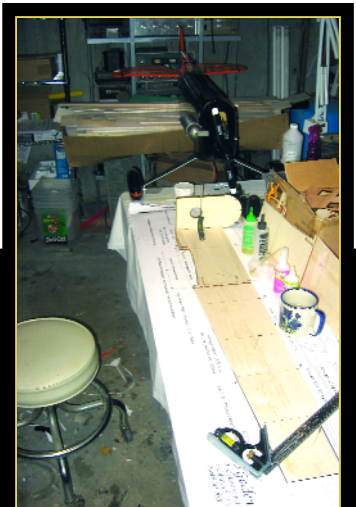
The former positions have been marked on the fuselage sides, and the firewall assembly has been epoxied in place.
