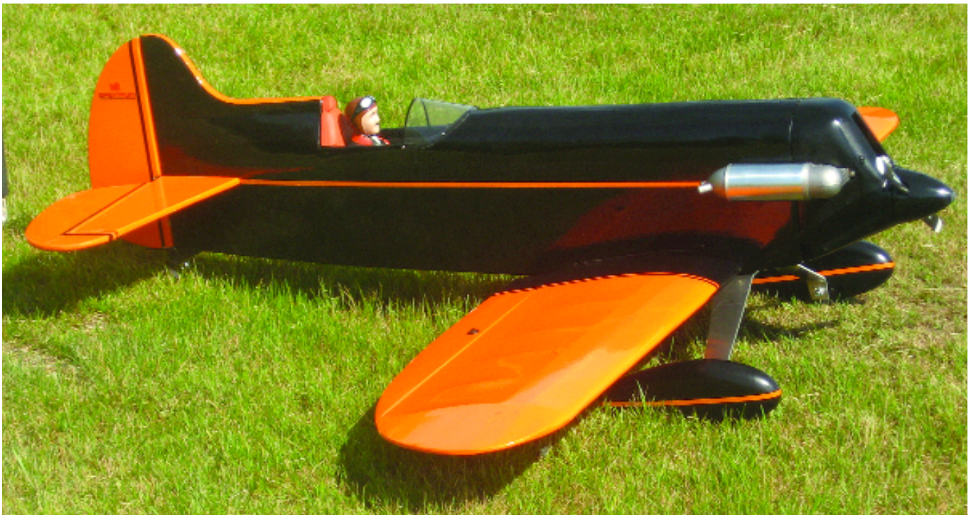
Stock Sig Four-Star 120 wheel pants complete this sport model's 1930s racing look. The long and tall fuselage offers good knife-edge performance.
