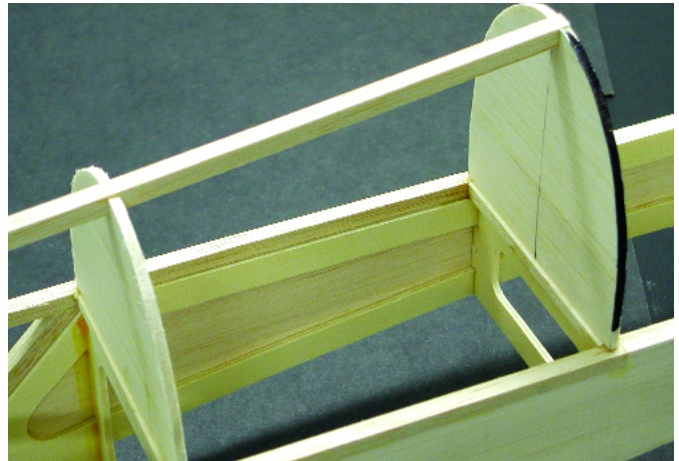
A good technique for making sure the formers are properly shaped before sheeting is to mark with Magic Marker and use a sanding bar to rub down high spots.
