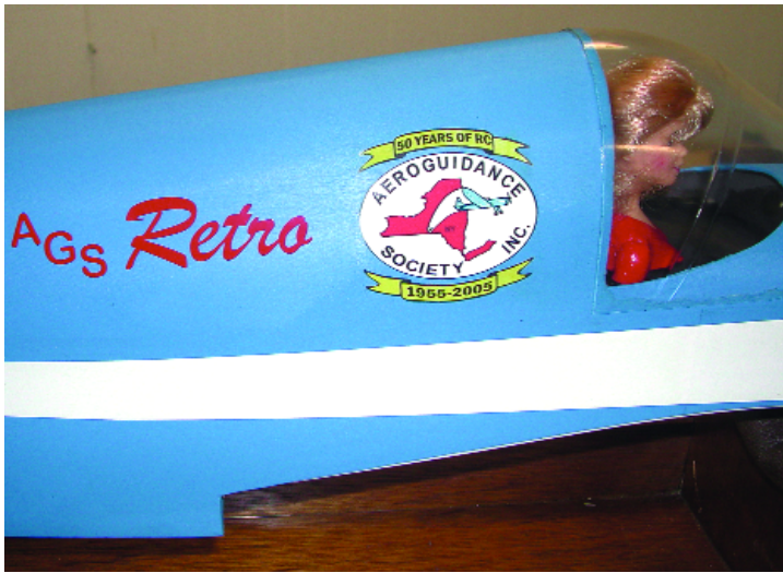
A Sig Four-Star I.20 (kit RC65) canopy was trimmed to a pleasing fit. It houses a doll bust from the local craft store.
