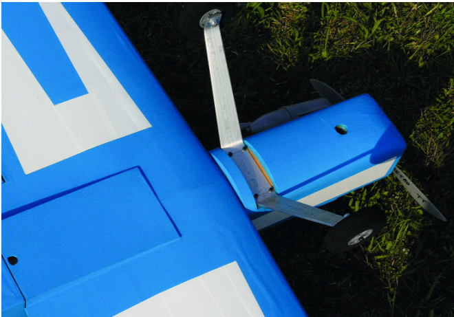
Just one 1/4-20 bolt is needed to secure the wing. The aluminum gear is good for rough fields.
