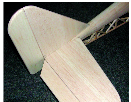
Above: The tail-feather parts are built up with \frac{1}{4} square balsa sticks that are sheeted with a \frac{1}{16} balsa skin.
