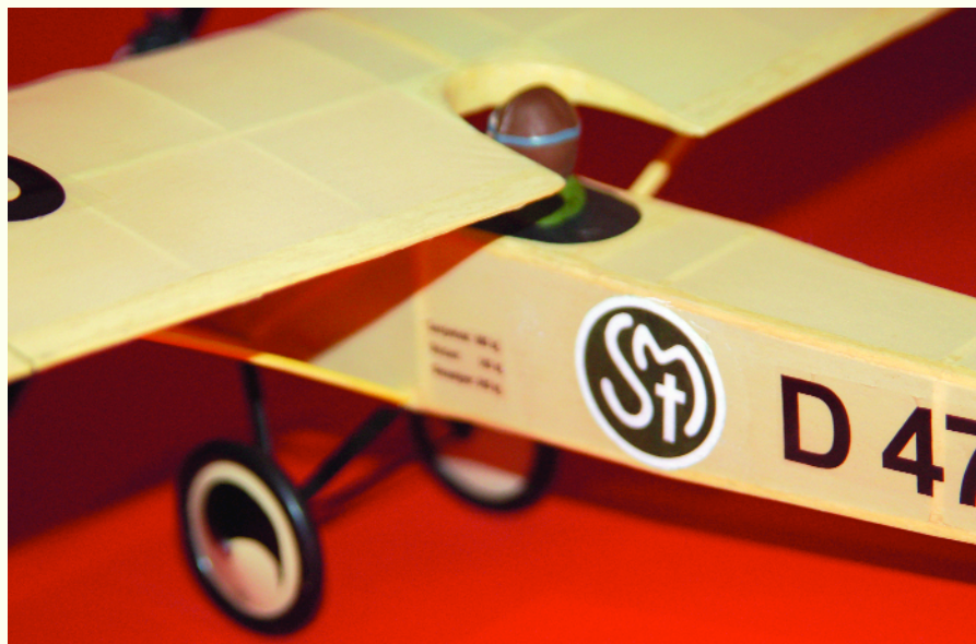
Any lightweight film-type covering, such as silkspan, or tissue-type materials can be used. A Williams Brothers 1/12th scale racing pilot bust was cut down to fit and painted.
