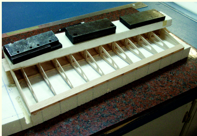
The LE shells are joined to the wing panels and are held in place accurately in the Lost Foam building cradle.
