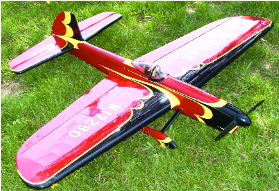
The Vulcan sports a fantastic finish. Bill used modeling dope for the base coats. Automotive polyurethane clear was applied over the top and rubbed out.
