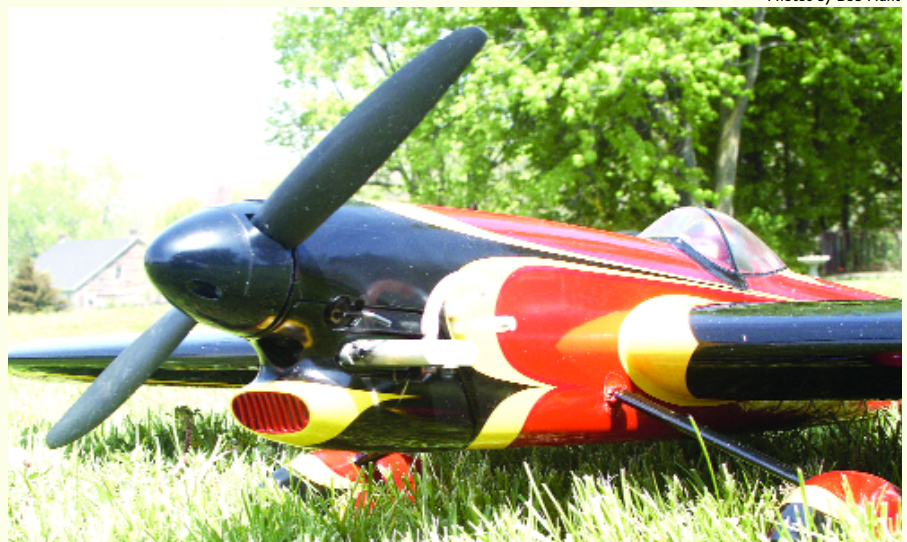
Bill tried several engines in the Vulcan, and he settled on the popular, powerful Aero Tiger .36. Notice the "tongue" muffler and the lightweight Hobby Lobby plastic spinner.
