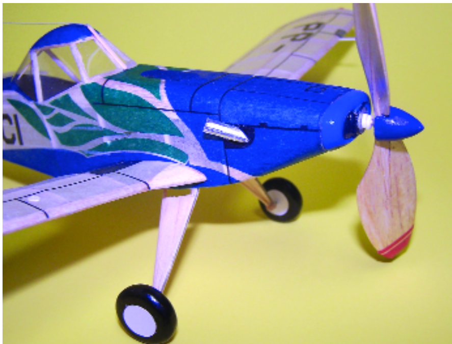
Nose-area details include soft-balsa wing-root fairings and exhaust pipes made from paper-backed aluminum foil. The back of the propeller is carved away for nose clearance.
