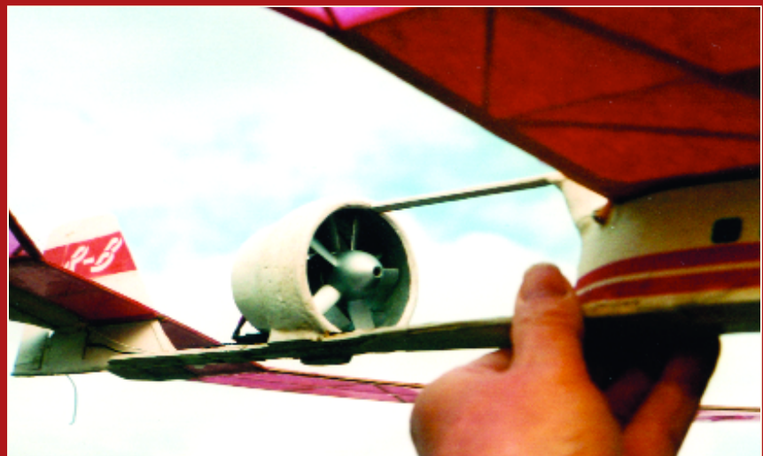
The second choice for power is to install a GWS 40 ducted-fan unit. The wide CG range allows this option.
