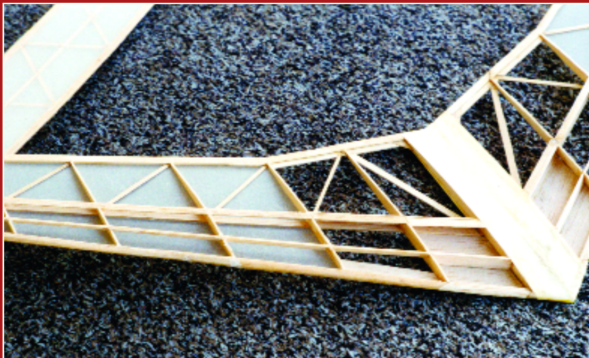
Notice the shear webbing between the ribs in the center-section. This adds considerable strength with a small weight penalty.
