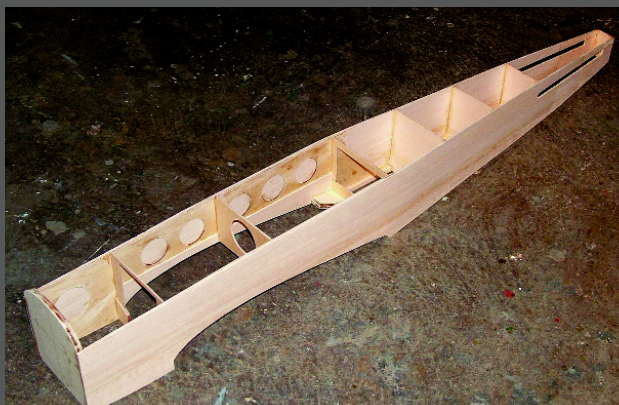
The fuselage assembly is basic. The sides and all the bulkheads are shown in place.
