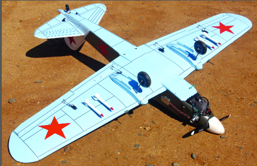
The bottom of Lou's Stormovik shows the location of the "ordnance." Notice the flap and aileron servo placement.
