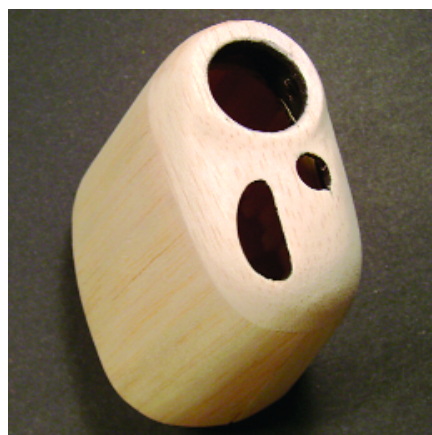
The cowl is framed and sheeted, and the nose block is installed. Notice the cooling holes.
