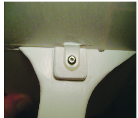
A closer look at the attachment, which is made with a Du-Bro 2 x 3/8 button-head screw (item 525).
