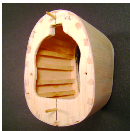
The rear of the cowl shows alignment dowels, two screw attach holes, and the motorstick clearance opening.
