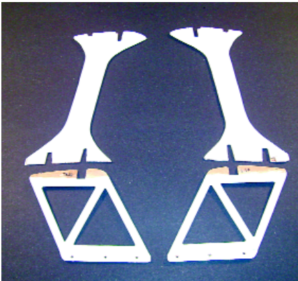
Cabane struts and wing struts (I-struts) completed and painted, ready for assembly. All struts are laminated with 1/64 plywood and balsa.
