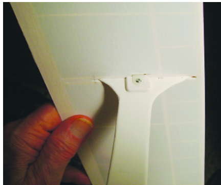
Bottom of right-hand upper wing, with I-strut installed. Shown is light-plywood pad attached to strut and Goldberg nylon strap (item 290).
