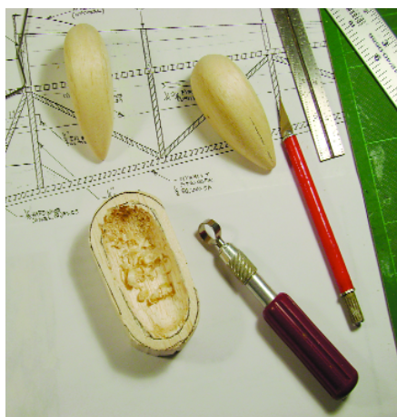
Use an X-Acto router to hollow out the nose block (just like scooping ice cream).
