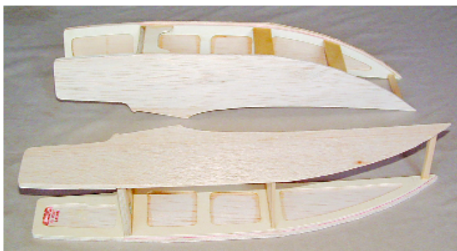
Doublers are glued to the nacelle sides and then the firewall and former F-2 are glued in place. Then the second side is added, along with firewall brace, rear spreader, and hatch mounts.
