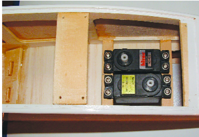
The throttle servo and optional aileron servo are screwed to hardwood mounting rails, and then the rails are fitted and glued into the nacelle.
