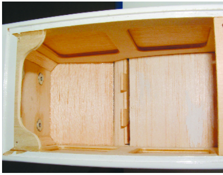
The nacelle is glued to the wing bottom, and F-I is glued to the back of the LE to anchor the nacelle.
