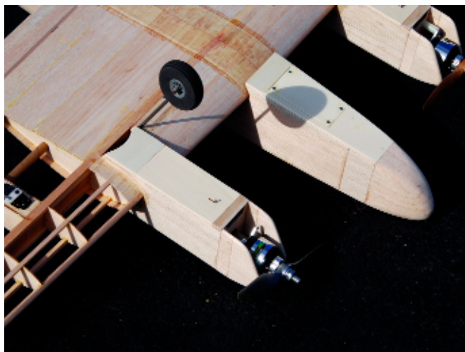
A bottom view of the completed airframe shows the nacelle with its bottom hatch in place.
