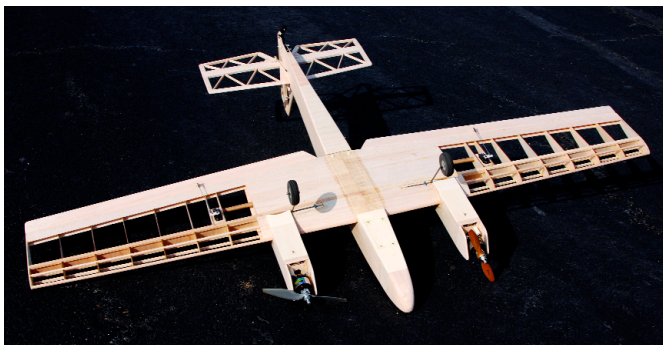
The bottom of the unfinished airframe reveals the exceptionally light structure. There is not too much sheeting!
