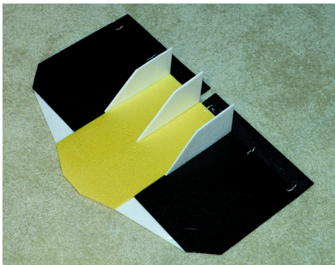
Foamy 5 in the test-glide phase. Weight is added to the nose and elevons are adjusted until it glides well. Mark the location on the wing bottom and use it as a safe starting point for the first flight.
