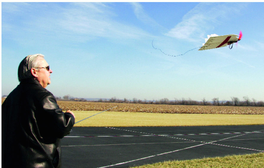
Foamy 1 launches nice and stable. Servos sticking through the wing's bottom give a good holding point for launching. They are inadequate for holding higher-power Foamys.
