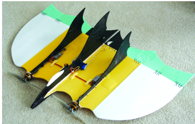
Twin Foamy was an experiment in using twin motors. Although it uses Jeti brushless outrunners, it would fly well with small GWS IPS geared motors.
