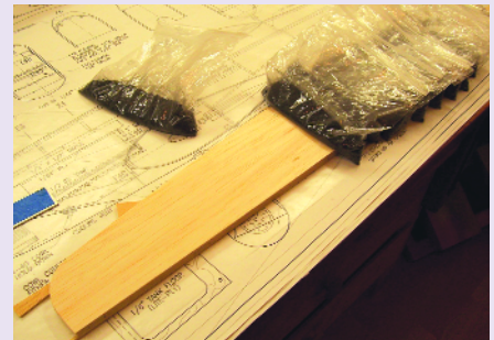
The bottom stabilizer sheeting is epoxied on, and lead shot in baggies holds it down.
