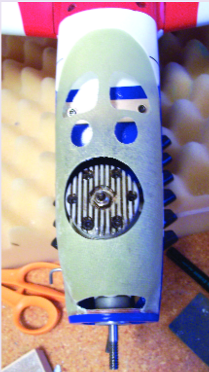
A second fiberglass cowling was made for an engine change to the Magnum .53 on the author's first Mustang.
