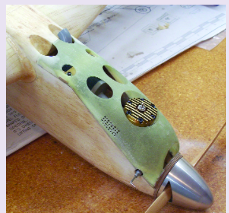
The finished fiberglass cowl has adequate vents to allow hot air to exhaust from the cowl.
