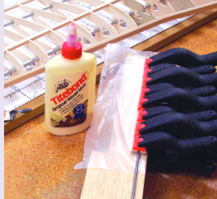
Landing-gear mounting blocks are laminated from 1/16 plywood and 1/8 plywood strips.
