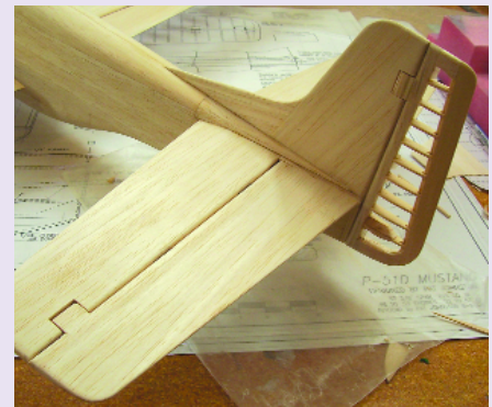
The completed tail reveals the balance tabs on the elevators and rudder. This adds realism.
